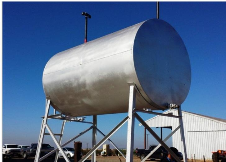
*"Freshly repainted tank with unapproved vents, no emergency venting, unapproved hose shutoff, unapproved tank for its use. Lack of labels and emergency venting indicates no UL listing for this tank." – Hank Moore, Merced County Fire Marshal*
