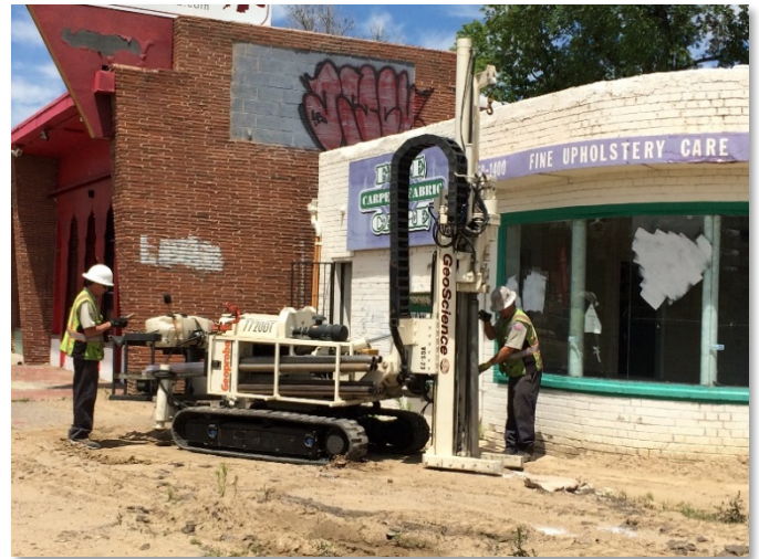
Direct-push soil sampling in a former tank basin can be conducted when tanks have been removed.
