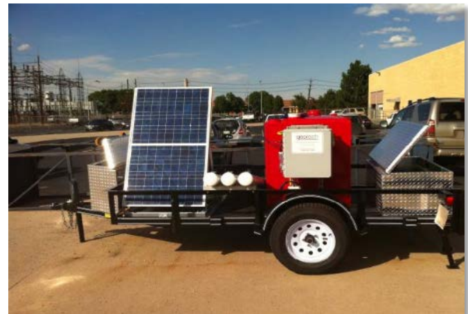
Utilization of a solar-powered remediation system is an example of a Green BMP.
