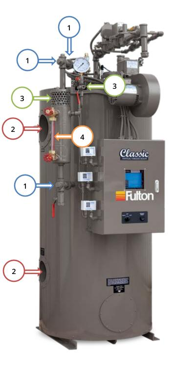
1 Cross tees must have the plugs removed to ensure there is an unobstructed opening
