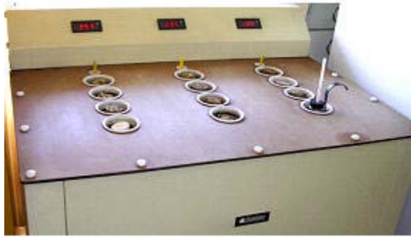
Cloud Point Analysis and two cloud point vials showing cloud point on the right.
